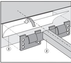
■ Position and attach the spring clips ① and support bars ② with strong, double-sided tape ③.
